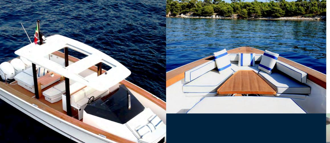
Another design feature is adding telescopic roof pillars and moving glass panels to create a convertible cabin. This allows the boat to be used either fully open or closed for privacy and comfort during bad weather.
