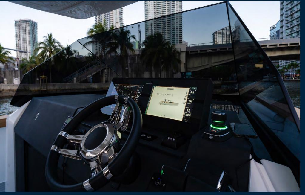
Intuitive steering system for multi-engine boats that places steering, as well as throttling and shifting, at your fingertips. The joystick provides "360-degree control," enabling you to move your boat sideways, forward, backward, diagonally or spin on its own axis.
